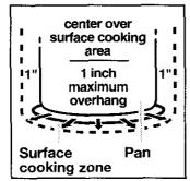
cooktops, especially radiant glass. Canners with rippled or ridged bottoms do not allow good contact with the surface.
